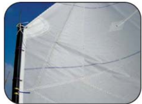
Right sprit tension. A little wrinkle perpendicular to the sprit is ok.
