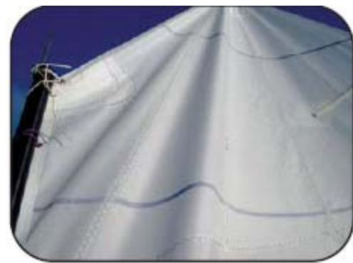
Wrinkle shows too much sprit tension
